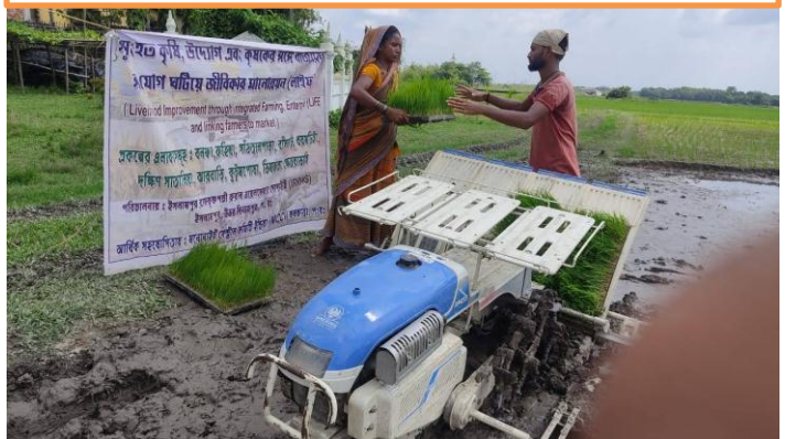
Paddy seedlings being transplanted by Paddy Transplanter machine by IRRWS at Ruhia Village of Islampur Block
